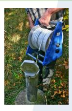
Water level meters are part of the standard equipment for the ascertainment of ground water levels. These mobile units are characterised by their simple, fast and solid acquiring of water level. With the variety of available models, you have the possibility to select the appropriate unit according to your individual requirements in cable length or operating convenience.
