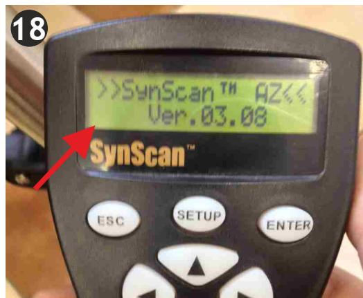
**EN** If both cables are connected properly, the hand controller starts operating. A beep will notify you of this.
