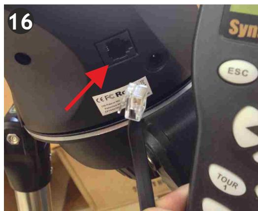
**EN** RJ-4 connector of the hand controller cable goes into the mount.
